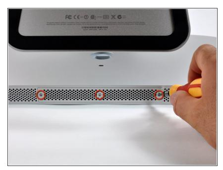
Like earlier iMacs, the RAM slots are hidden beneath an access door at the bottom of the iMac. A Phillips #2 screwdriver makes quick work of the three screws.
