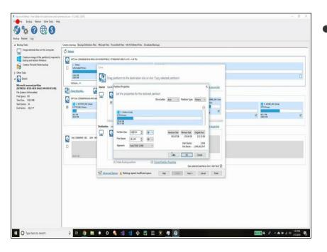
but what you are aiming for is to bring over the C drive from the old SSD to the new one and open up the partition to the maximum allowable size that still leaves room on the drive for the old boot files, other back up files, and all the other drives you want copied over
