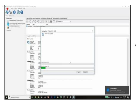
Here we are finishing up the cloning of the old drive over to the new drive with Macrium Reflect. Once the drive is successfully cloned all that is left is to open up the machine and physically uninstall the old drive and reinstall the new drive in it's place. Since you cloned the boot drive, the new SSD should boot up with no issues once installed
