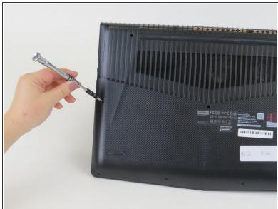
You will need to remove thirteen 6.5mm screws (with a Phillips #00 screwdriver) from back of the laptop to make it possible to pry off the back cover.
