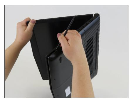
Turn the laptop on its side and use an opening tool, spudger, or similar plastic device to pry the back cover off. Prying off the back cover can be a little bit challenging but just stick with it until you hear the tabs pop open and then you should be able to pry the rest of it off.
