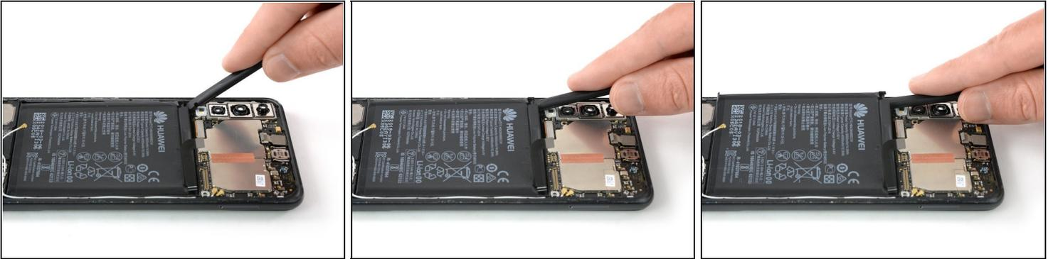
ⓘ In case you have trouble to pry up the battery the adhesive may not be loose enough. You can apply some isopropyl alcohol under each corner of the battery and allow it to penetrate for about two minutes to help weaken the adhesive.
