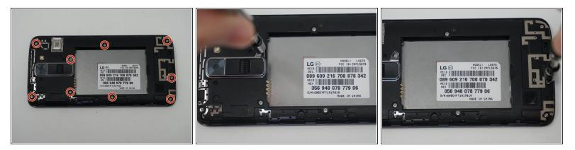
Remove the nine 2mm JIS #00 screws from the mid-frame.
