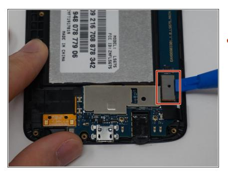
Disconnect the flex cable from the motherboard with the iFixit opening tool.
