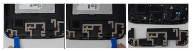
• Using an iFixit opening tool, remove the antenna extender located at the bottom.
