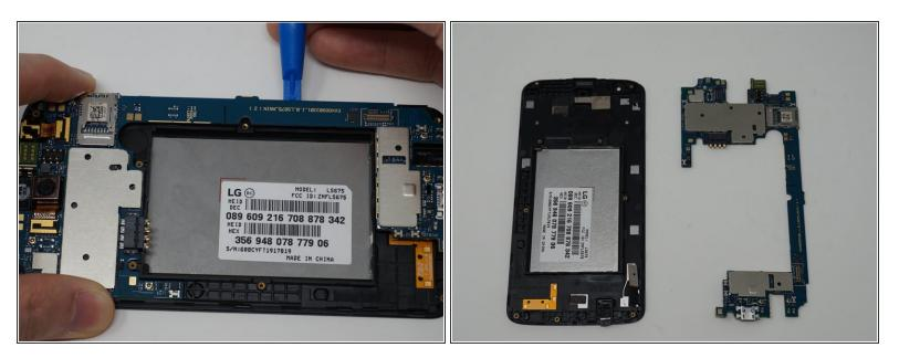
• Use an iFixit opening tool to separate the motherboard and the display.
