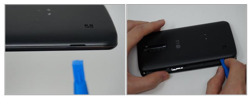
Using an iFixit opening tool, gently pull outward on the cutout on the bottom left corner of the phone to remove the back cover.
