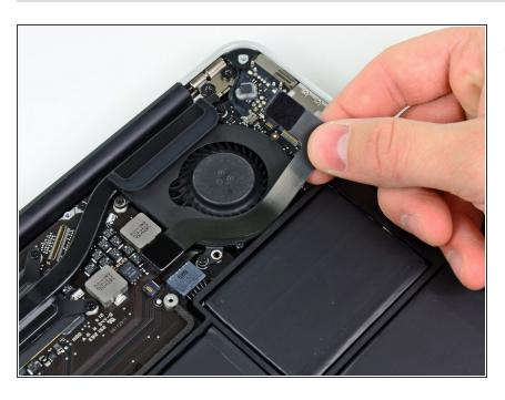
Peel the I/O board cable up from the adhesive securing it to the fan.
