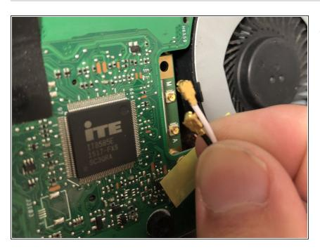
Disconnect the two wires connected to the network card.
