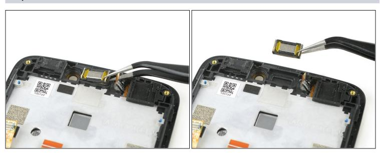
• Use a pair of tweezers to carefully grab and remove the earpiece speaker.
