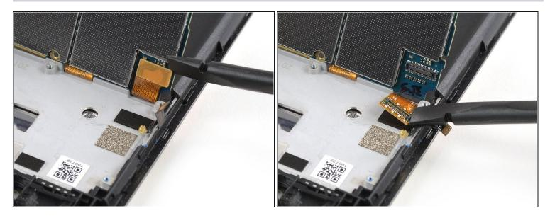
• Use the edge of a spudger to pry up and disconnect the display flex cable from the motherboard.
