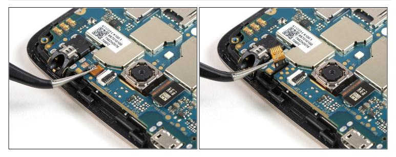
• Use a pair of tweezers to pull the flex cable out of the ZIF connector.
