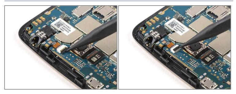
• Use the tip of a spudger to open the flap of the ZIF connector next to the headphone jack.
