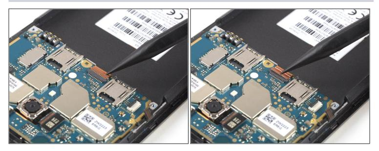
• Use the tip of a spudger to open the interconnect cable ZIF connector by lifting the brown flap.
