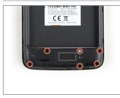
Remove the six 3.1 mm Phillips #00 screws securing the daughterboard cover.
