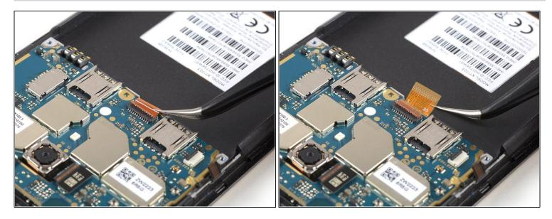
• Use a pair of tweezers to pull the interconnect flex cable out of the ZIF connector.
