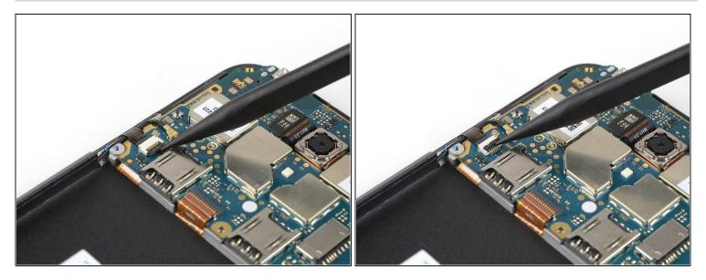
• Use the tip of a spudger to lift the latch on the power and volume button ZIF connector.
