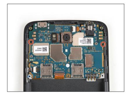
Remove the two 3.2 mm Phillips #00 screws securing the motherboard.
