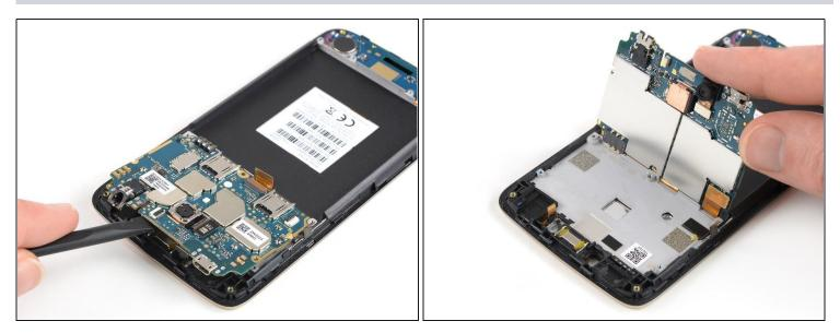
▲ Don't try to remove the motherboard all the way yet. The display flex cable is still connected to its rear side.
