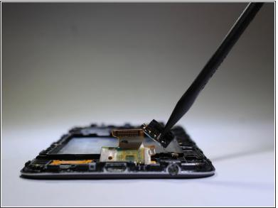
• Use the point of a spudger to pry the headphone jack out of its recess in the display assembly.
