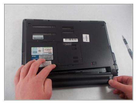
Now you can remove the battery while continuing to hold the right battery lock in the unlock position.
