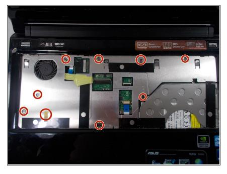
Remove the nine 5 mm screws using the Phillips #0 screwdriver.
