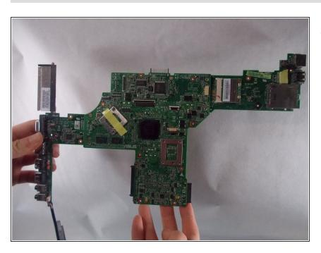
Lift the motherboard out of the laptop and remove it from the device.
