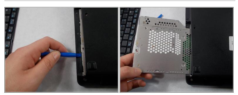
• Use the iFixit opening tool to remove the cd drive on the left of the laptop.
