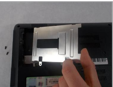
Slide the hard drive away from the SATA connector and remove the hard drive from the device.
