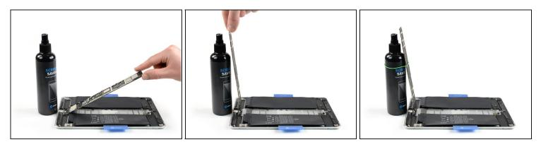
⚠ In this step, don't fold back the logic board to more than a 100° angle. Some connectors are still attached to it and can be damaged.
