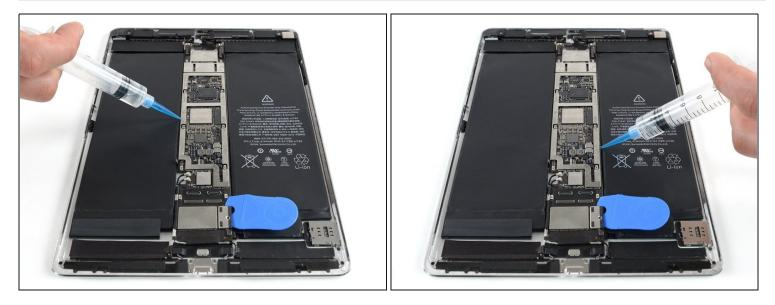
(i) The adhesive that holds down the logic board is very strong. To remove the board, you must first weaken the adhesive using either a solvent, or heat.
