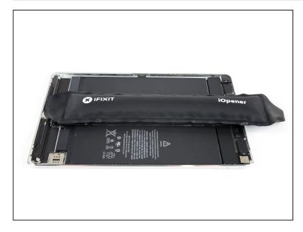
• Apply a <u>heated iOpener</u> to the EMI shield to loosen the adhesive beneath. Apply the iOpener for at least two minutes.
