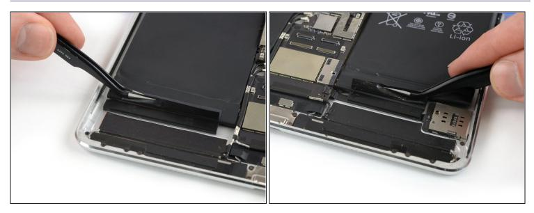
• Peel up the black adhesive strip at the bottom edge of each battery cell, if they didn't already come off during the prying procedure.
