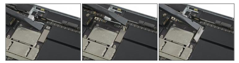
• Use the edge of a spudger to pry up and disconnect both the right interconnect cable and antenna cable, and gently fold them out of the way.
