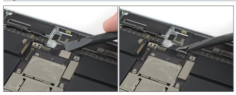
• Use the edge of a spudger to pry up and disconnect the microphone array cable.
