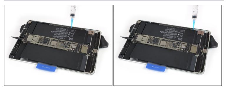
• Continue separately applying solvent at the remaining two <u>adhesive strip locations</u>. Allow it to penetrate for several minutes to help weaken the adhesive.
