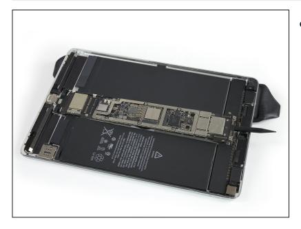
Elevate the left side of the iPad (long edge nearest the headphone jack) by placing an iOpener underneath, so that the iPad lays down at an angle.
