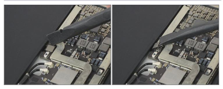
• Use the edge of a spudger to pry up and disconnect the cable for the Smart Connector, and fold it out of the way.
