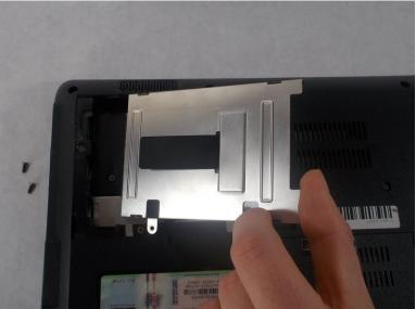
Slide the hard drive away from the SATA connector and remove the hard drive from the device.
