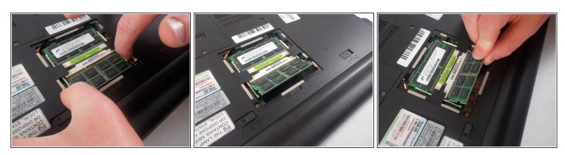
• Pull the clips toward the chassis of the computer. The RAM will pop up and can easily be removed.
