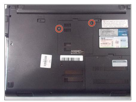
Flip computer over and unscrew the two 5 mm screws using the Phillips #0 screwdriver.
