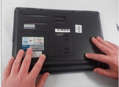
Identify the two slide locks below the battery. Slide them outward towards the unlock symbol. You should see a red mark that indicates that the battery is unlocked and is ready for removal.
