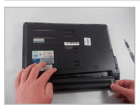
Now you can remove the battery while continuing to hold the right battery lock in the unlock position.
