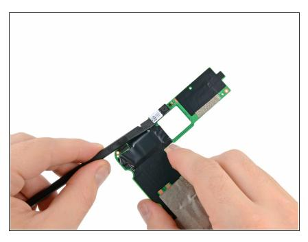
Use the flat end of a spudger to pry the front-facing camera straight off of its socket on the motherboard.
