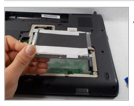
Carefully lift and remove the disk drive keeping in mind the port. To install replacement and reassemble your device, carefully follow these instructions in reverse order. When doing so, make sure to observe precautions for handling electrostatic sensitive devices.
