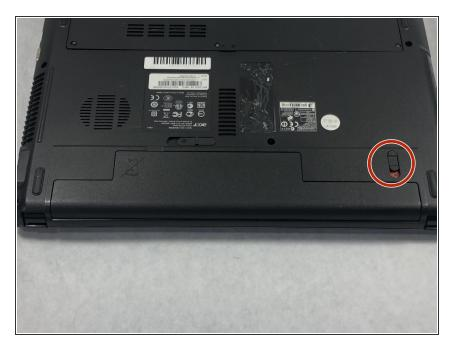
Flip the lock latch to unlock battery.
