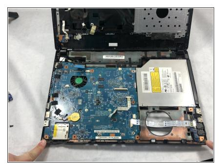
Using the prying tool to remove the bottom of the laptop.
