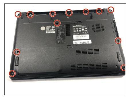
Remove all 12 screws from the backplate using a Phillips #0 screwdriver.
