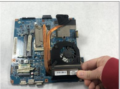
Unscrew the 6 screws that hold the fan to the motherboard using the same screwdriver.
