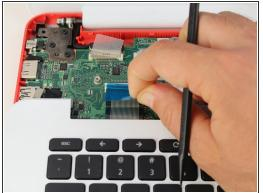
• Disconnect the two ZIF connectors by prying up the locking bar with a spudger and removing the ribbon cable.
