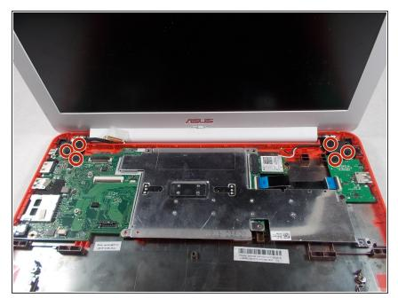
Use a Phillips #0 driver to remove the six 5mm screws on the top right and left display hinges.
