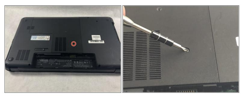
• Using a Phillips #0 screwdriver, loosen the service door screw.
