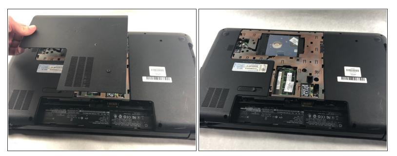
• Lift the service door up and away from the device.
