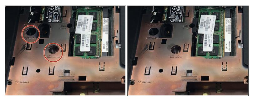
Insert the pointy end of a spudger into the two keyboard release holes and press down to disengage the keyboard from the device.
