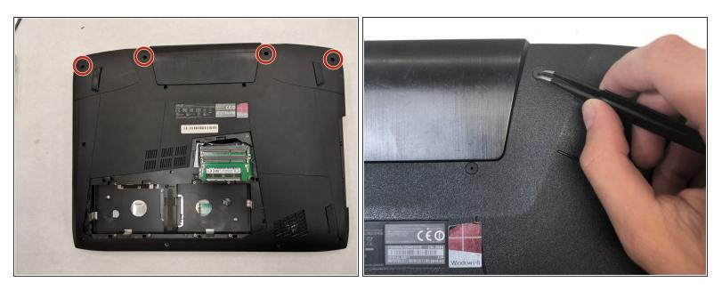
• Use a pair of tweezers to remove the top four rubber stoppers found on the bottom of the laptop.
