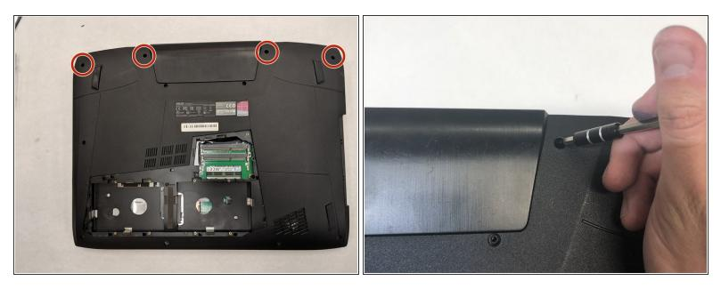
• Use a Phillips 1 Screwdriver to remove the top four 8.5 mm screws.
