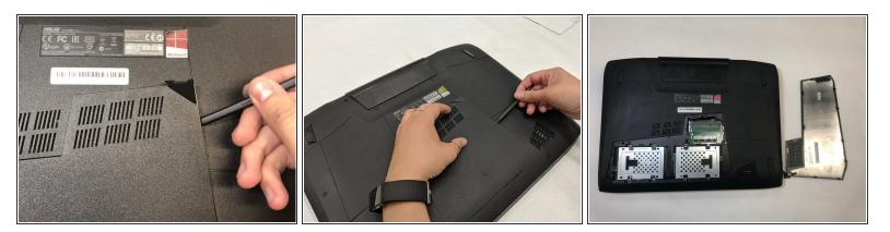
• Use the standard spudger to remove the back center panel.
