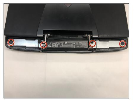
Use a Phillips 1 Screwdriver to remove the four 6.8 mm screws underneath the back panel.
