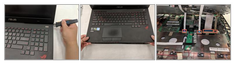
• Use a metal opening tool to pry the keyboard from the base of the laptop.
