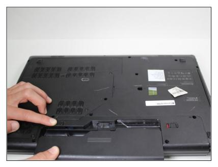
Hold the battery release switch in the unlocked position and remove the battery.
