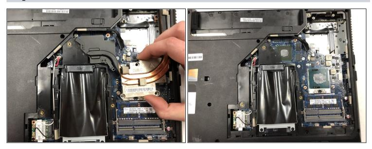
• The heat sink needs to be rotated counter-clockwise slightly to allow space for removal.
