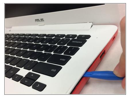
Separate the plastic case from the keyboard at the seam by using a plastic opening tool.
