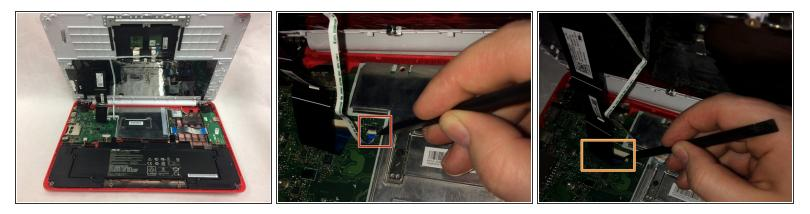
(i) The small and wide ribbon cables connect the keyboard to the motherboard.
