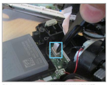
Connect the light bar cable using your fingers. Make sure it is fully pushed down and that is plugged in the right way.
