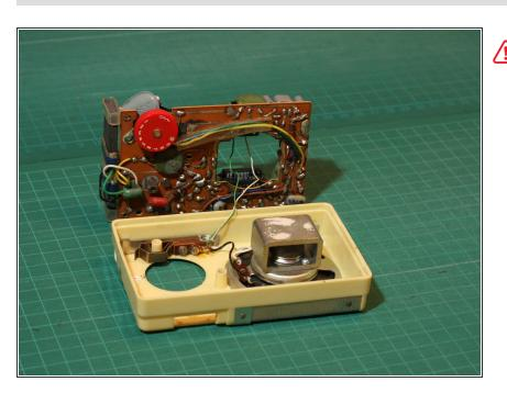
Set the circuit board beside the case, being careful not to damage the thin wires going to the earphone jack and speaker.
