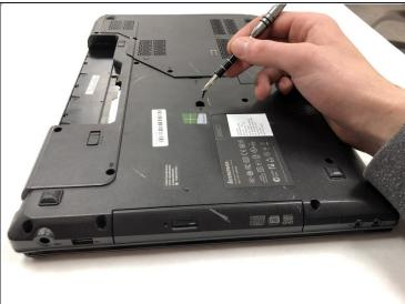
• Remove the 8.5 mm holding screw using a Phillips #1 screwdriver.
