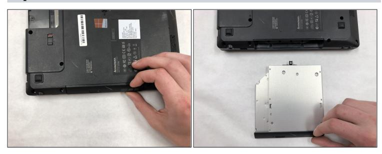
• Pull the optical drive from the device
