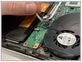
Use the plastic opening tool to disconnect the ribbon connector.
