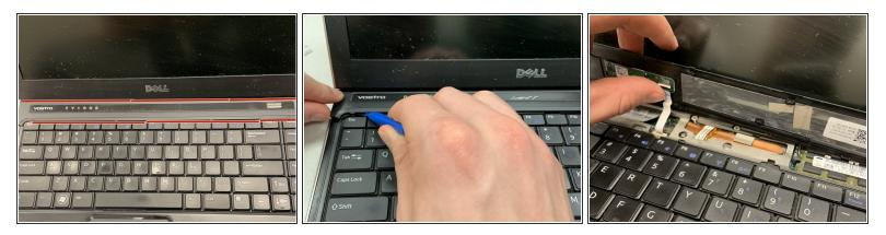
• Wedge the plastic opening tool around the seam of the notification panel to pop it off.
