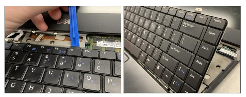
• Use the plastic opening tool to pry the keyboard out of the laptop.
