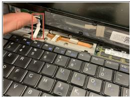
Disconnect the ribbon connector by using the plastic opening tool.
