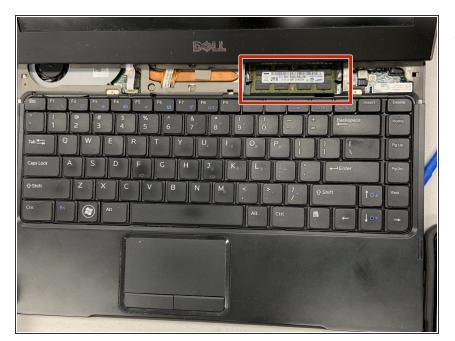
Remove the panel to reveal the RAM.
