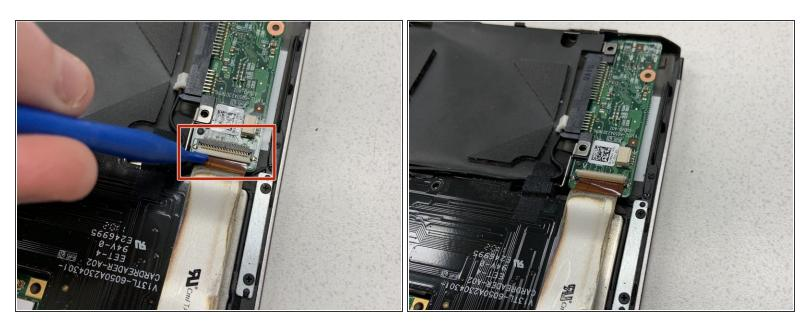
• Use the plastic opening tool to flip the ribbon connector up.
