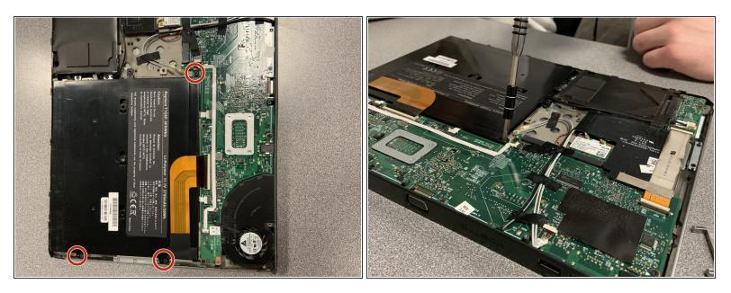
• Remove the three black 3.9 mm Phillips #1 screws holding the battery in place.
