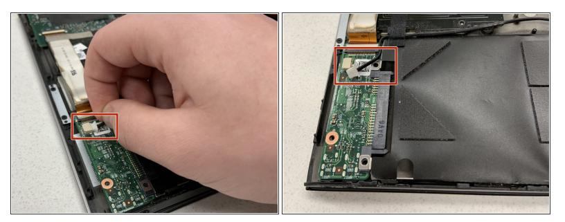
• Disconnect the white plug on the top left corner of the sound card.
