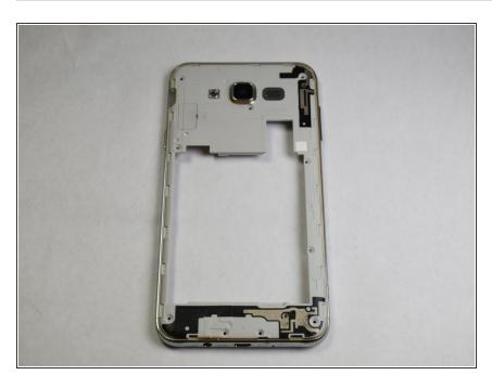
Once your device's back has been disassembled, grab the panel that has the volume buttons.
