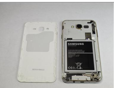
Remove the back of the device by pulling on the tab in the top left.
