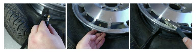
• Insert the new stem up through the rim. Use the diagonal cutters to help pull the stem into its seated position. There will be an audible pop when it is in correctly.
