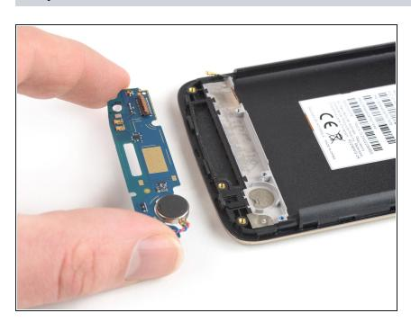
Remove the daughterboard including the soldered-on vibration motor. To reassemble your device, follow these instructions in reverse order.
