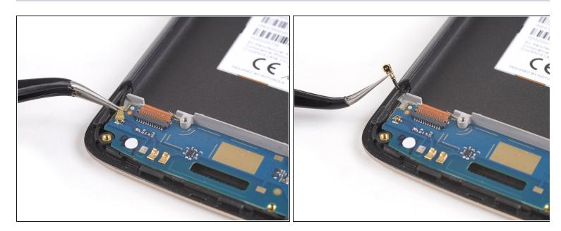
Disconnect the antenna cable and fold it out of the way.
