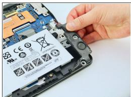
Use a plastic spudger to gently coax the cable connecter sideways from the motherboard and the left speaker. When disconnected, remove speaker.
