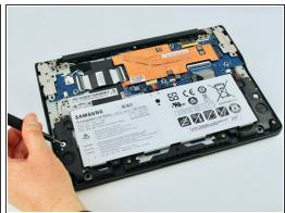
Remove one 4.9mm silver screw from each speaker with a Phillips #00 screwdriver.
