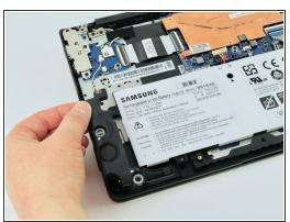
Use a plastic spudger to gently disconnect the cable connecter from the daughterboard and the right speaker. Remove the speaker.
