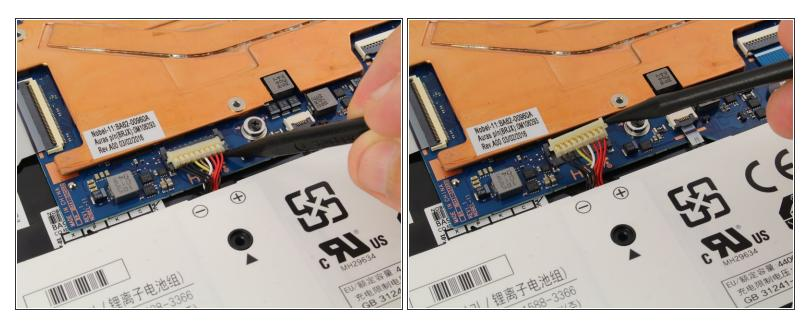
Disconnect the battery from the motherboard by prying upwards on the cable connector with a spudger.
