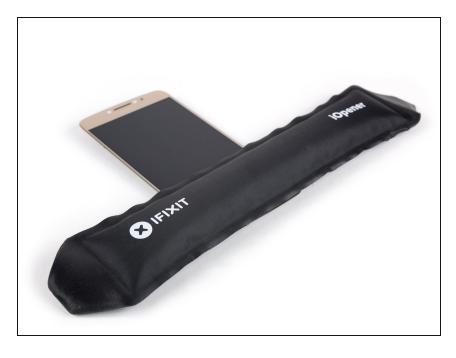
Apply an iOpener to the bottom edge of the screen for about a minute to loosen the adhesive beneath the fingerprint sensor.
