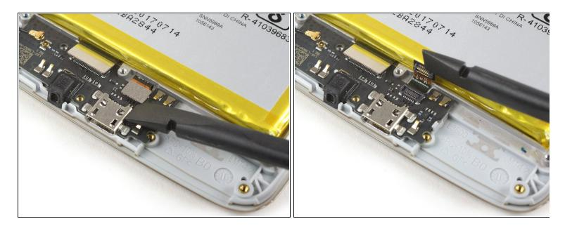
• Use the edge of a spudger to pry up and disconnect the fingerprint sensor flex cable.
