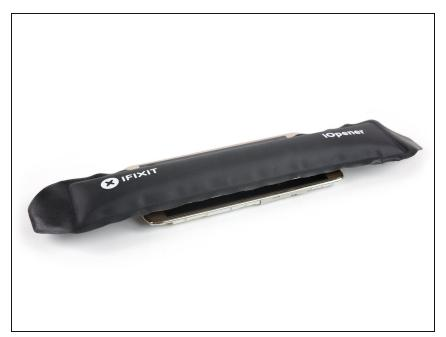
Prepare an iOpener and apply it to the display for at least two minutes to loosen the adhesive underneath.
