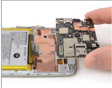
• Grasp the motherboard by the top corners and remove it by lifting up and pulling it carefully out of its recess.
