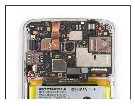
Remove the two 2.9 mm Phillips screws.
