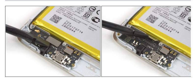
• Use the edge of a spudger to pry up and disconnect the interconnect flex cable.
