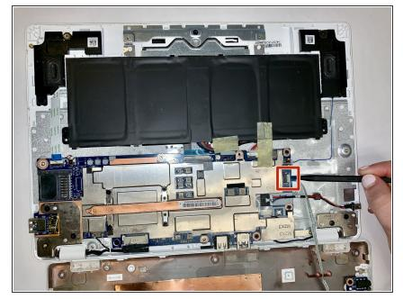
Use the pointed side of the spudger to disconnect the headphone jack cable from the motherboard and completely remove the bottom cover.
