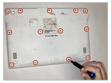
Flip the computer over and use a Phillips #0 screwdriver head to remove the 13 2.5 mm bottom cover screws.
