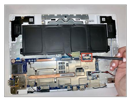
Use the pointed side of the spudger to disconnect the battery cable from the motherboard.
