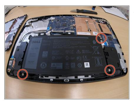
Remove the 3 battery screws with a phillips #00 screwdriver.
