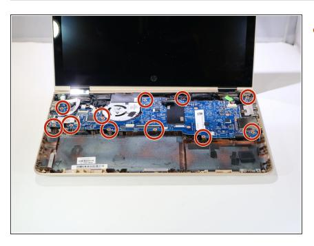
Remove eleven 2.0 x 4.6mm screws using the Phillips 00 Screwdriver
