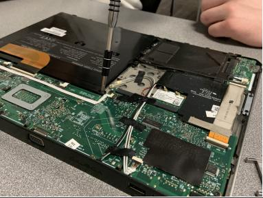
Remove the three black 3.9 mm Phillips #1 screws holding the battery in place.
