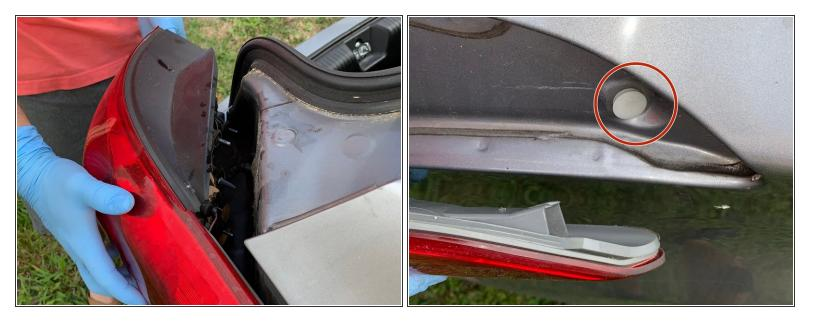
Once the wires are disconnected facing the bumper, firmly grasp the entire plastic casing of the tail light and pull directly towards your hips in order to not catch the hidden clip located on the side of the car near the end of the tail light casing.
