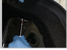
You will then use your 10mm socket to remove three nuts, careful not to strip the screw to ensure easy replacement.
