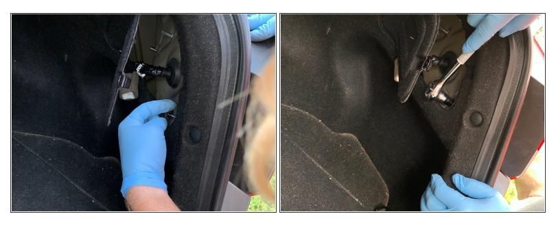
Next you will need to screw on the three bolts used previously with a 10 mm socket making sure they are tight and secure.
