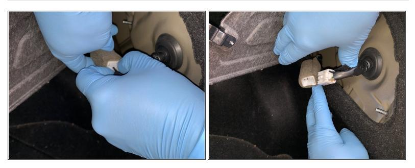
Once the bolts are removed, you will need to remove the wires connected to the bulb casing.
