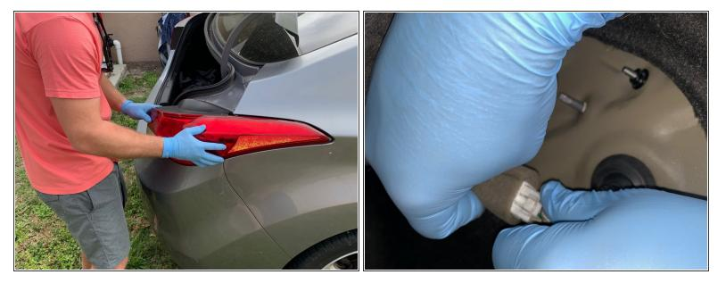
After you seal the bulb, you will then place the entire casing back into the bumper ensuring that the hidden clip mentioned earlier is attached. Then, re attach the wires, you should hear a clicking sound when wire is properly placed in socket.
