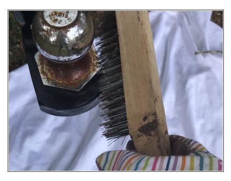
Apply the wire brush on any part of the hitch in order to brush off any excess rust or rust flakes.
