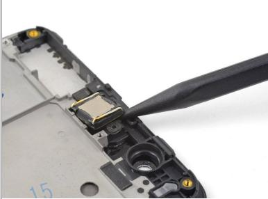
Insert the point of a spudger under the top right corner of the earpiece module and pry up, loosening the module from its recess.
