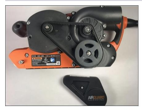
• Remove the timing belt housing.
