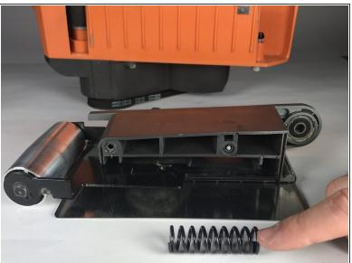
Remove and replace the spring (OD 14.47mm X 38.1mm).
