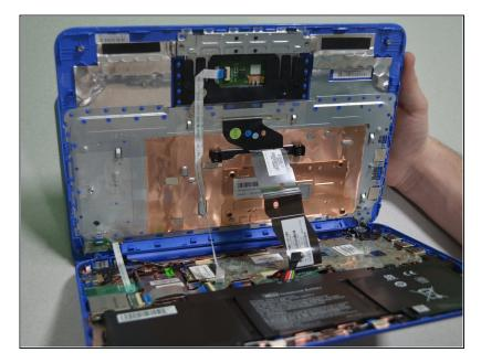
Lift the keyboard out of the laptop to remove it from the device.
