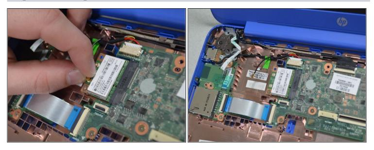
• Unplug the black wire attached to the wireless chip.
