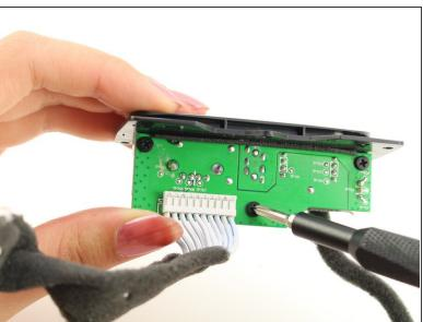
Remove the three 9mm Phillips #0 screws from the board.
