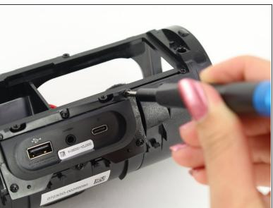
Remove the six 6mm Phillips #0 screws.
