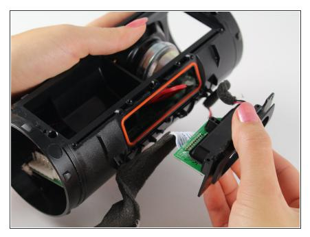
Remove the port bay from the device and place the device to the side.
