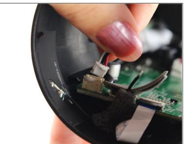
Remove the second connector on the opposite side by gently pulling it out.
