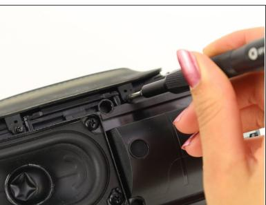
Remove the two 6mm Phillips #0 screws from either side to remove the port bay cover.
