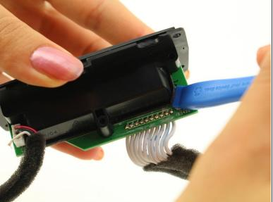
Using the plastic opening tool, lift the board from the port bay holder.
