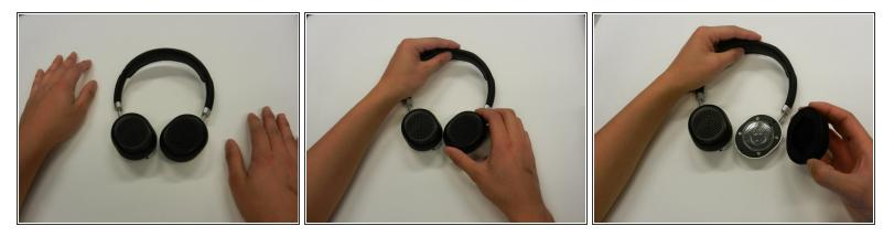
• Pull the cushion off of the desired side by gripping the top of the headphones and pulling the cushion off.
