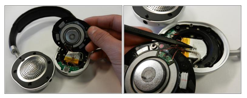
• Remove the tape attaching the thicker white wire to the battery. You may consider keeping the tape to reattach the wire later.
