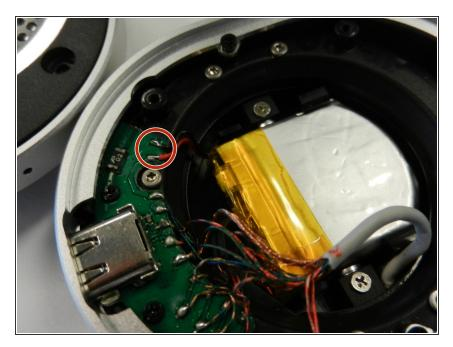
• Desolder the two wires circled here.
