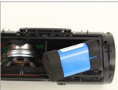
Remove the battery from the battery socket by gently pulling on it.
