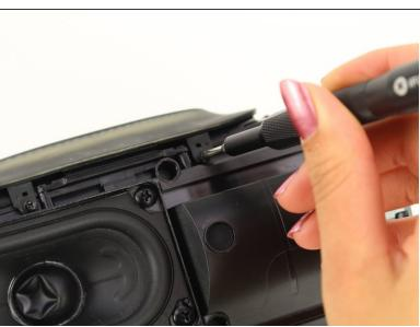
Remove the two 6mm Phillips #0 screws on the front side of the port bay cover.
