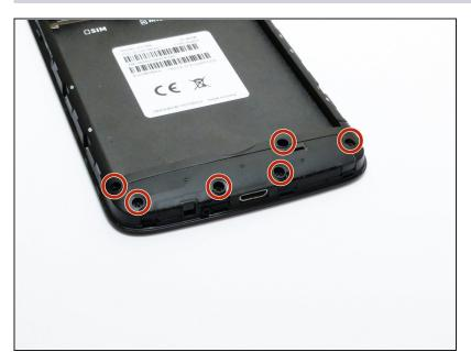
Remove the six 4mm screws from the bottom plastic cover with a Phillips driver bit.
