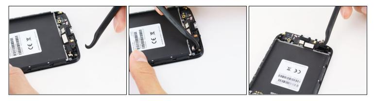
• Lift the vibrator out of its slot using the Halberd Spudger hook.
