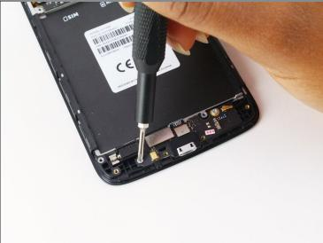
Remove the two 4mm silver screws holding down the charging port board with Phillips bit.
