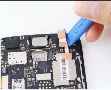
Detach the front facing cable ribbon connector using an iFixit opening tool and lift the camera out of position.
