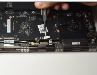
Pull out the ribbon cables from the opened connectors using the iFixit Tweezers to free up the motherboard.
