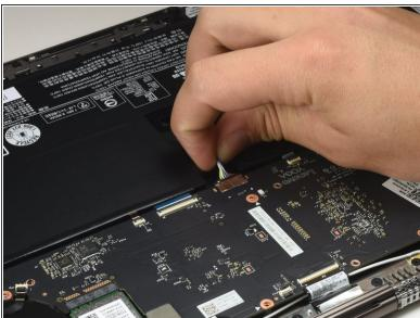
Disconnect the battery by pulling the ribbon wire grouping out of the top of the motherboard.
