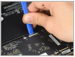
• Flip up the ten flat connectors holding the motherboard using the iFixit Opening Tool to free the motherboard.
