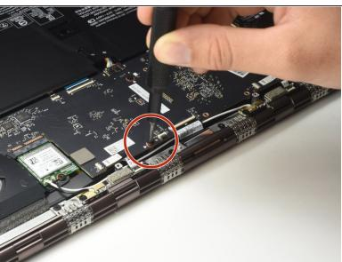
Remove the twelve 5mm Phillips #00 screws to loosen the motherboard.
