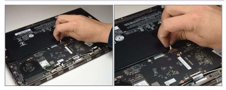
• Disconnect the battery by pulling the ribbon wire grouping out of the top of the motherboard.
