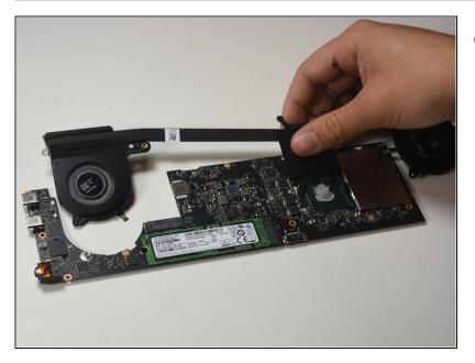
• Separate the fans from the motherboard to isolate it for replacement.
