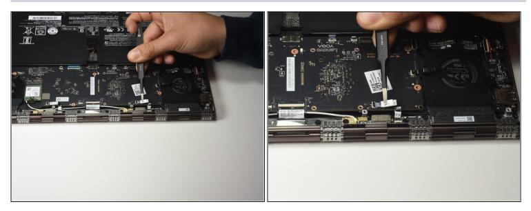
• Pull out the ribbon cables from the opened connectors using the iFixit Tweezers to free up the motherboard.
