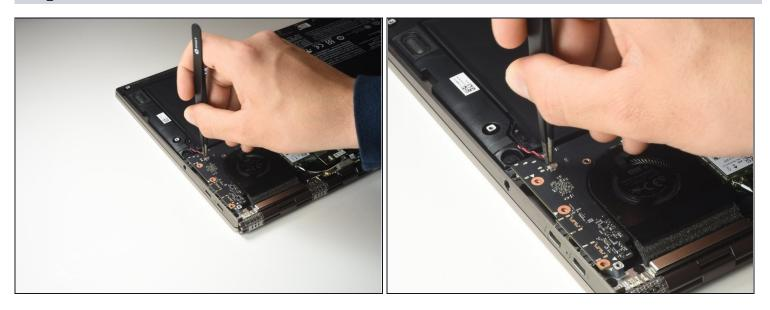
• Disconnect the red and black wire from the motherboard using the iFixit Tweezers.
