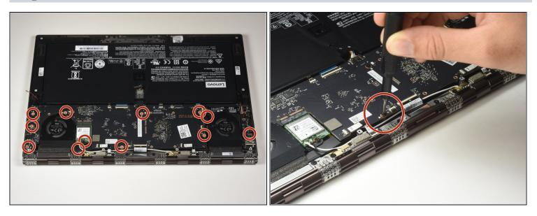
• Remove the twelve 5mm Phillips #00 screws to loosen the motherboard.
