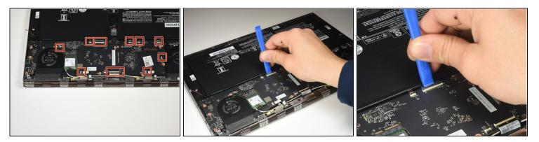
• Flip up the ten flat connectors holding the motherboard using the iFixit Opening Tool to free the motherboard.
