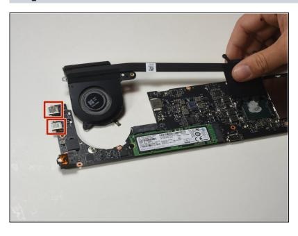
• Replace the motherboard to replace the USB-C ports.
