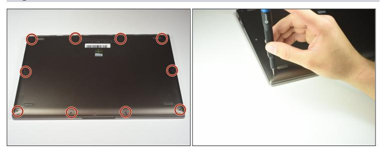
(i) Flip the device over to access the screws on the back cover.
